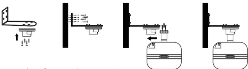
1. Join the L-frame and connector 1
