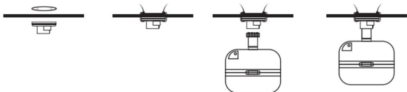
1. Fasten the round frame with the screws or strappings.
